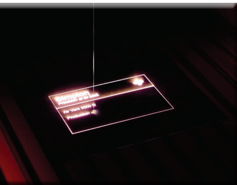
There are a variety of ways that metal marking can be achieved, including laser engraving. (Image courtesy of Trotec Laser)
